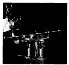
The unique feature of the Access-A-Bilt chemical reactor is the magnetic coupling device which allows the agitator shaft to be split near the top and the hinged head of the vessel to swing open like a lid. The reactors are constructed of stainless steel and can be supplied in sizes up to 100 gallons, with pressure ratings up to 250 pounds/sq. inch PE1
